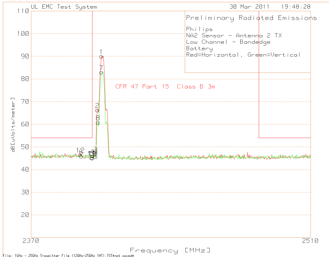
Figure 23 Radiated Band Edge Compliance Graph – Antenna 2
