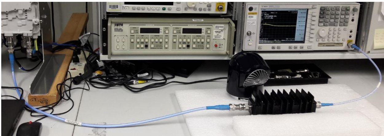
Photograph of 20MHz to 3GHz and 3GHz to 6GHz Test Setup
