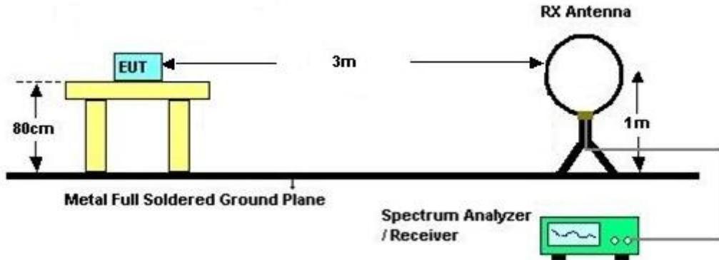
For radiated test above 30MHz
