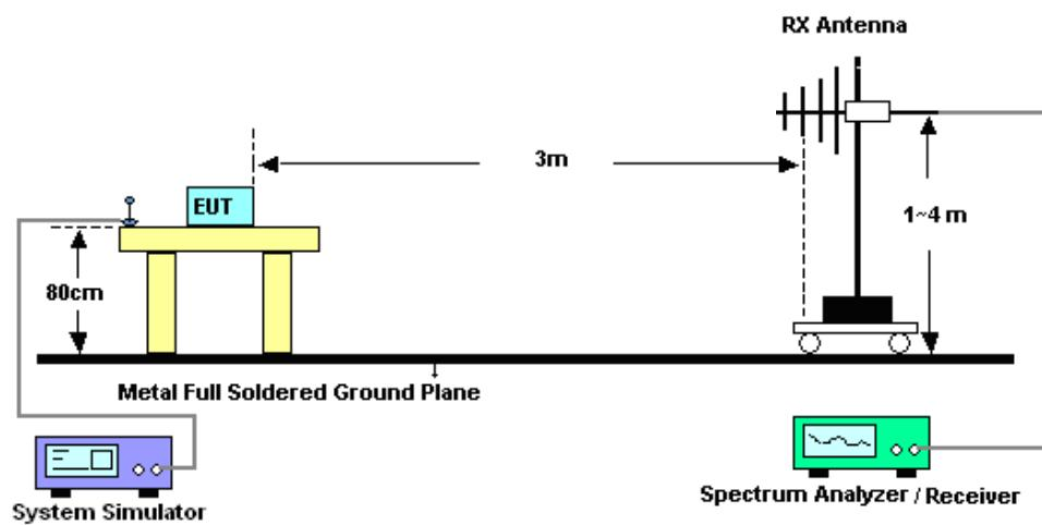
For radiated test above 1GHz
