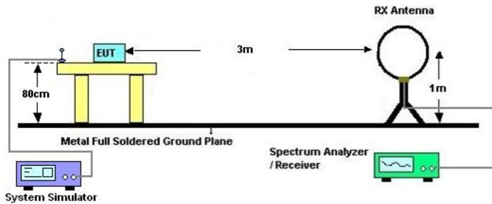
For radiated test from 30MHz to 1GHz
