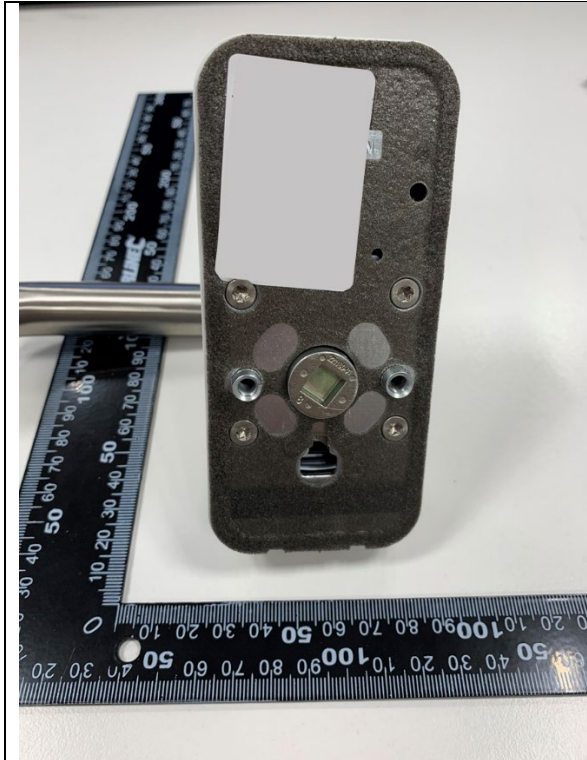
Photo 5: Back of the part of the lock located on the outside of the door.
