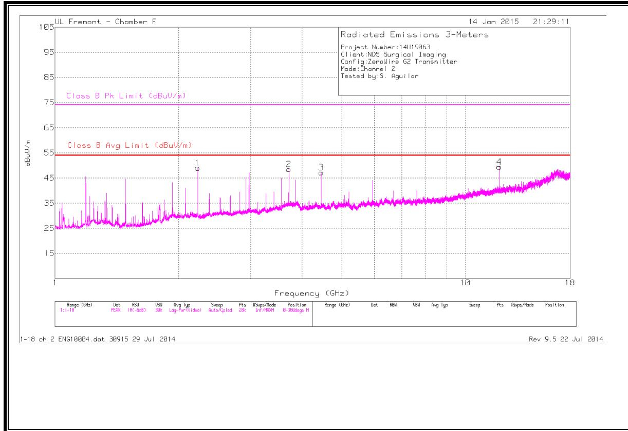
**CHANNEL 2 – TX SPURIOUS EMISSION 1-18 GHz (VERTICAL PLOT)**
