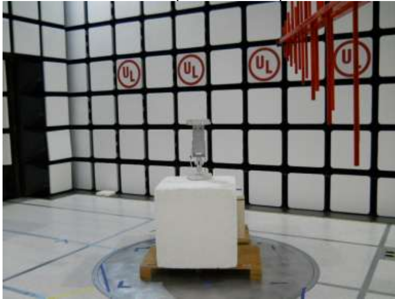
RADIATED FRONT PHOTO (BELOW 1 GHz)
