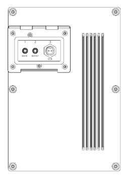
Audio and DC inputs are waterproof when the cover is securely closed.
