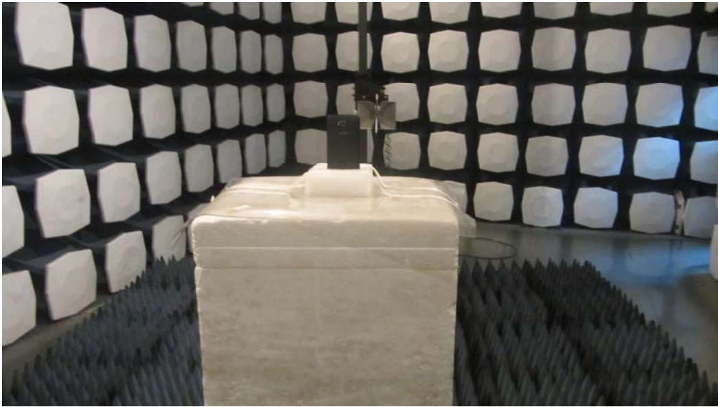
Picture 2: Radiated Spurious Emissions Test setup
