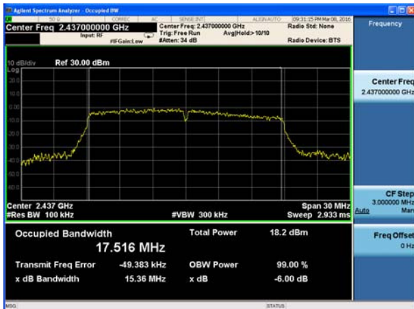
802.11n(HT20), Carrier frequency (MHz):2462
