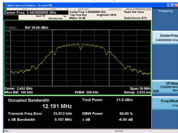
802.11b, Carrier frequency (MHz): 2462
