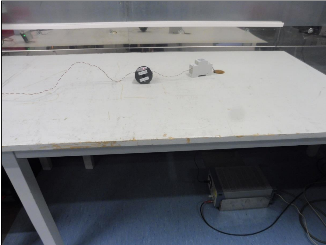
Photo 2: setup of radiated emission < 1 GHz
