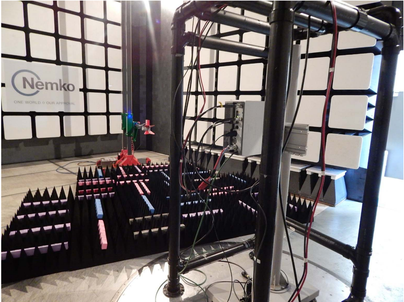
Figure 8.3-2: EUT Set -up for Radiated Compliance Testing
