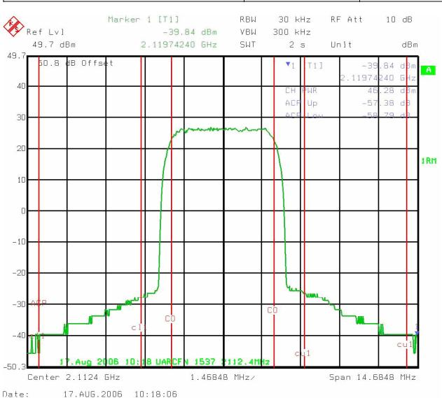
Test Result for QPSK on 2112.4MHz
