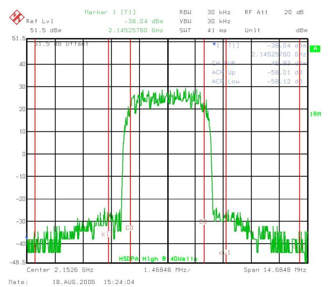
Test Result for 16 QAM on 2152.6MHz
