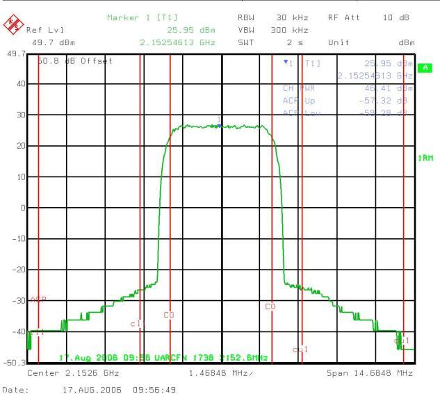
Test Result for QPSK on 2152.6MHz
