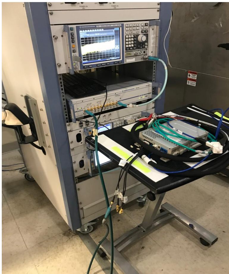
Figure C2: Conducted DUT Set up
