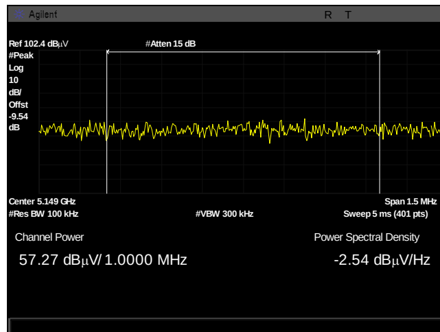
Plot 313. Undesirable Emissions, PK, 5150 bandedge, 23dBi, 30M, 5165M, power integration
