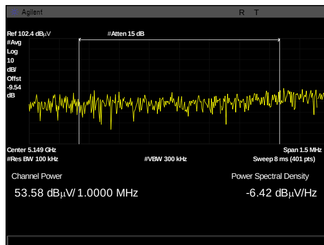
Plot 304. Undesirable Emissions, AVG, 5150 bandedge, 23dBi, 20M, 5160M, power integration
