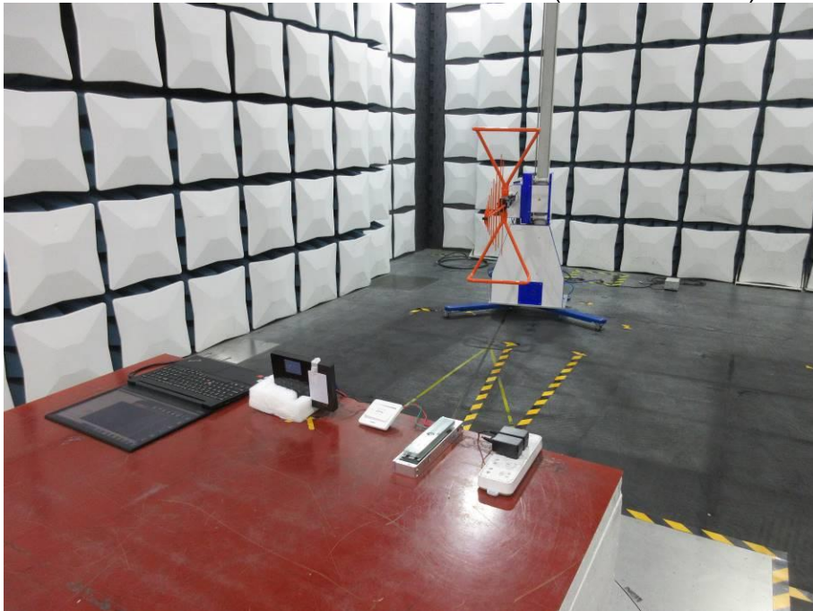
RADIATED RF MEASUREMENT SETUP (30MHz ~ 1 GHz)
