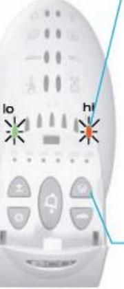
The ( hi ) flow red light on the water use indicator gauge will illuminate as soon as 2 or more faucets are opened fully creating a water flow of more than 9 ltrs min
