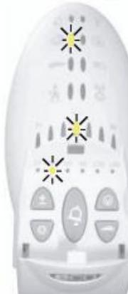
Following the 48 hour "set up" procedure the Waterminder will set to the Auto mode utilising the optimised time settings the system has recorded over the preceding 48 hours
