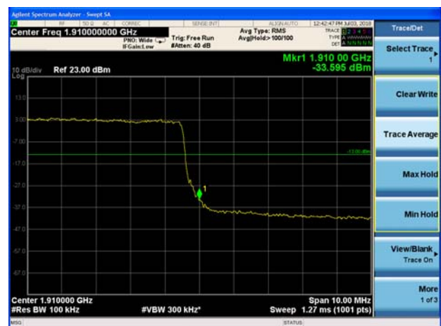
LTE Band 2 10MHz QPSK 100%RB CH-High
