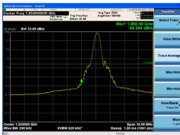
LTE Band 2 20MHz 16QAM 1RB CH-Low
