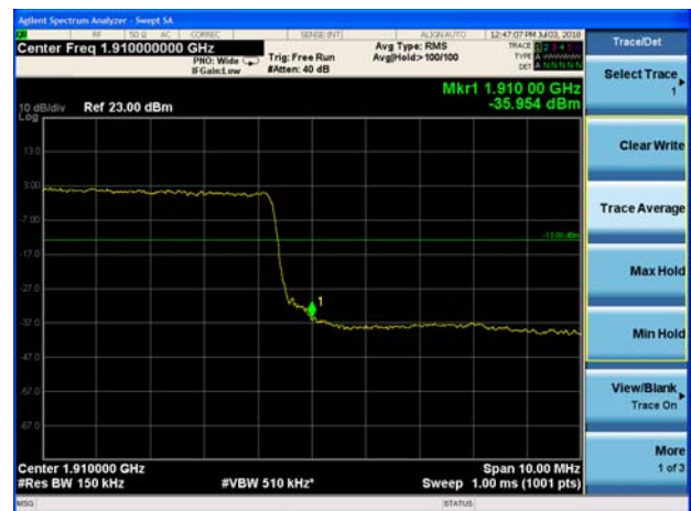
LTE Band 2 20MHz 16QAM 1RB CH-High
