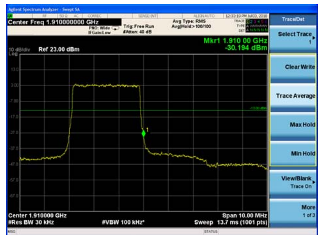
LTE Band 2 5MHz QPSK 1RB CH-High
