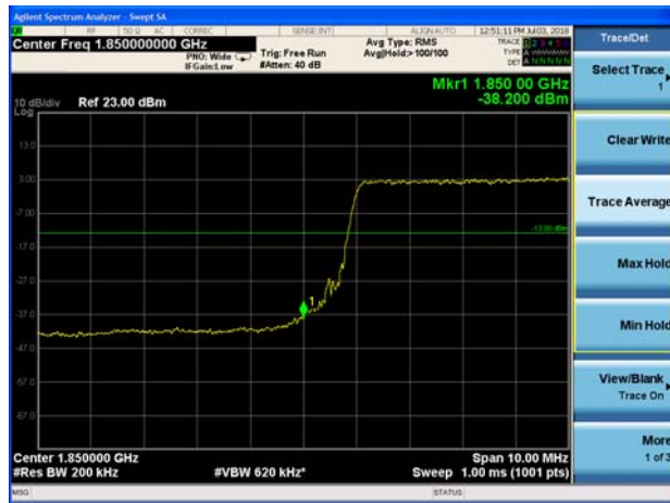
LTE Band 2 1.4MHz 16QAM 1RB CH-Low
