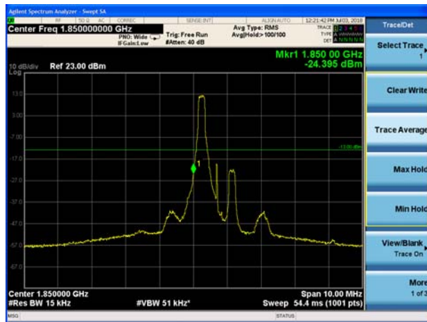
LTE Band 2 1.4MHz 16QAM 100%RB CH-Low
