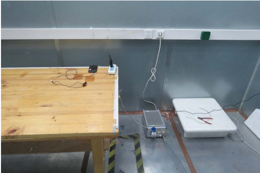
Picture 3 Conducted Emission Test Setup
