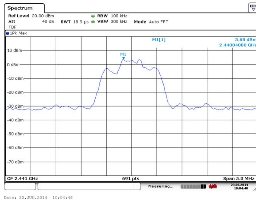
Fig. 25 Conducted Spurious Emission ( \pi/4 DQPSK, Ch39, 2.441GHz)
