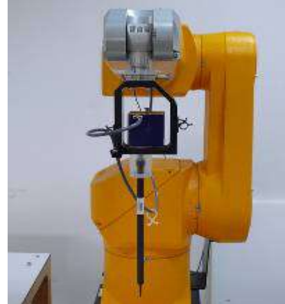
Figure 5-3. ES3DV3 E-field probe
