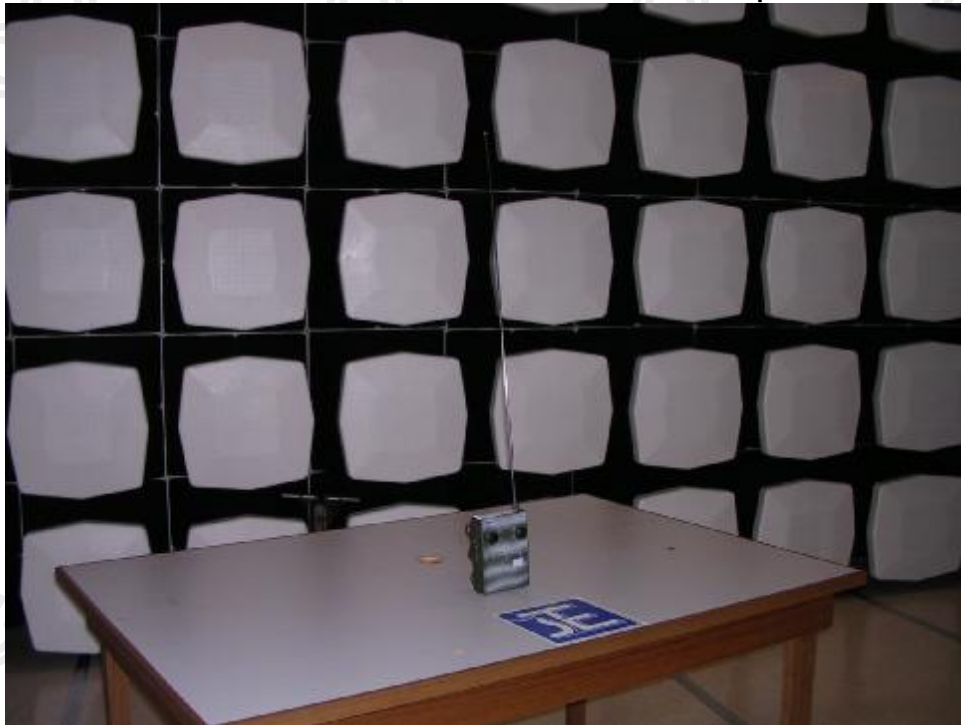
Measurement of Radiated Emission Test Set Up
