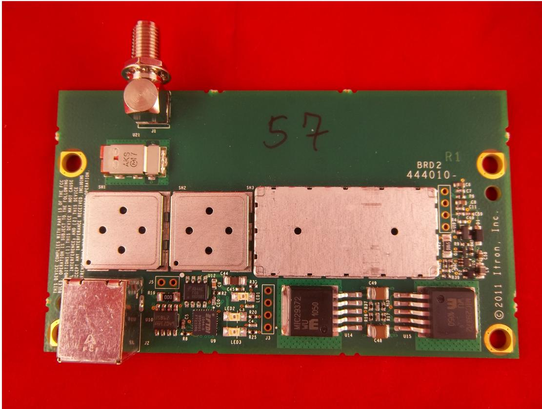
Figure 1 Itron ITR9002 module, FCC ID: SK9ITR9002
