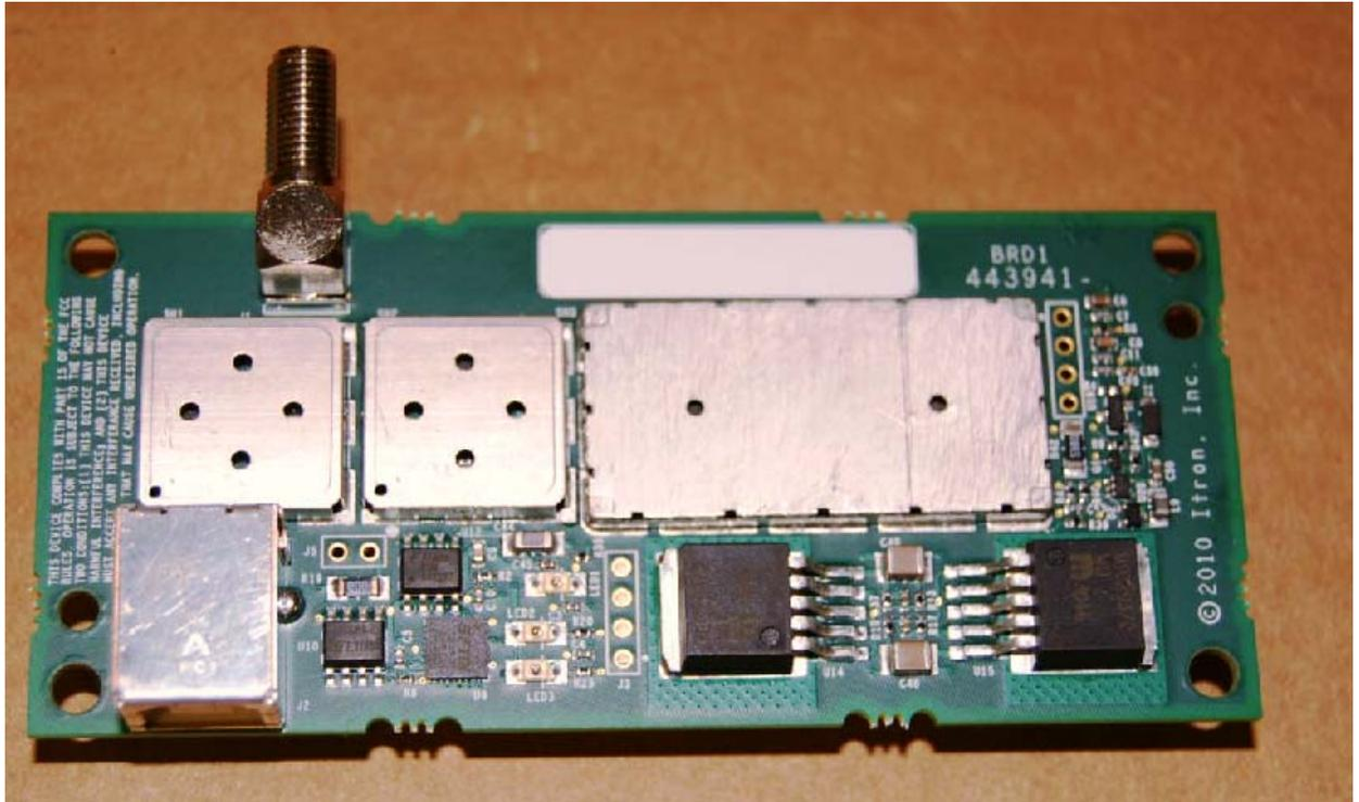
Figure 1 Itron ITR9002 module, FCC ID: SK9ITR9002
