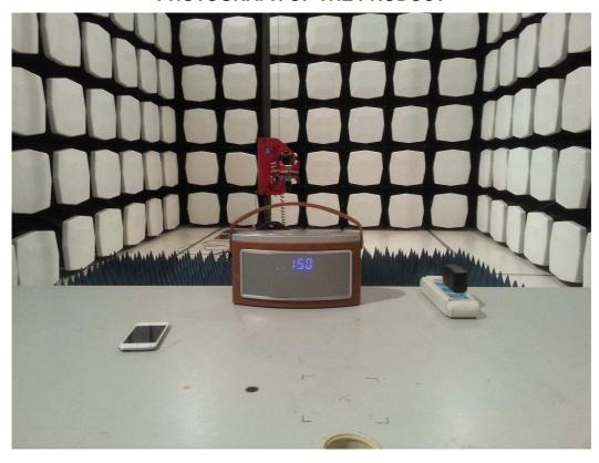
**MEASUREMENT OF CONDUCTED EMISSION TEST SET UP**
