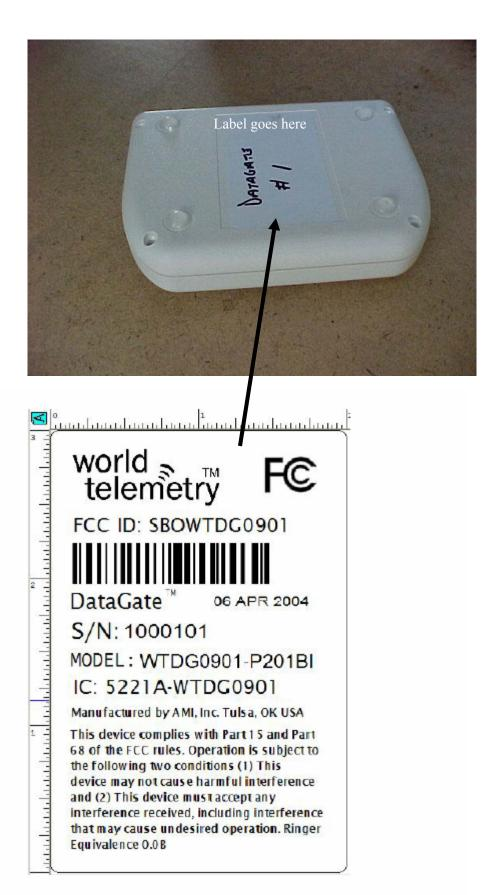
Label to be placed a the bottom of the DataGate
