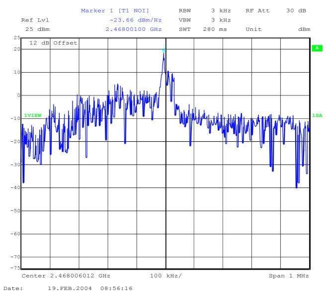
Power density: -23.66 dBm/Hz = +6.34 dBm / 3 KHz
