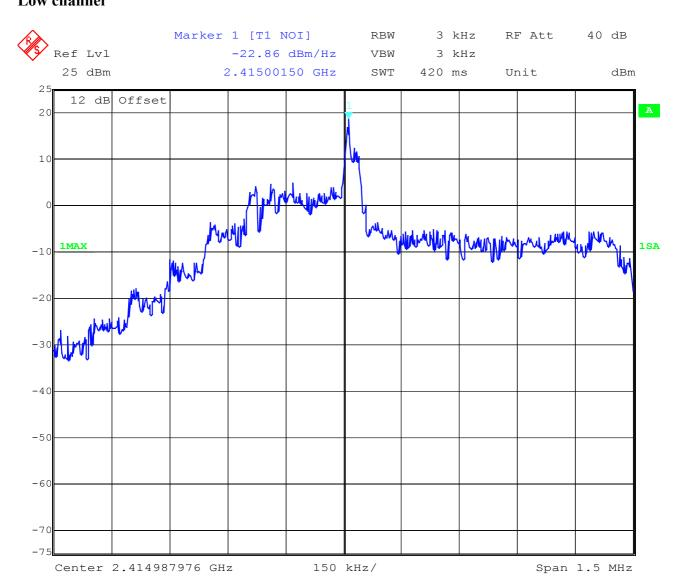
Power density: -22.86 dBm/Hz = +7.14 dBm / 3 KHz
