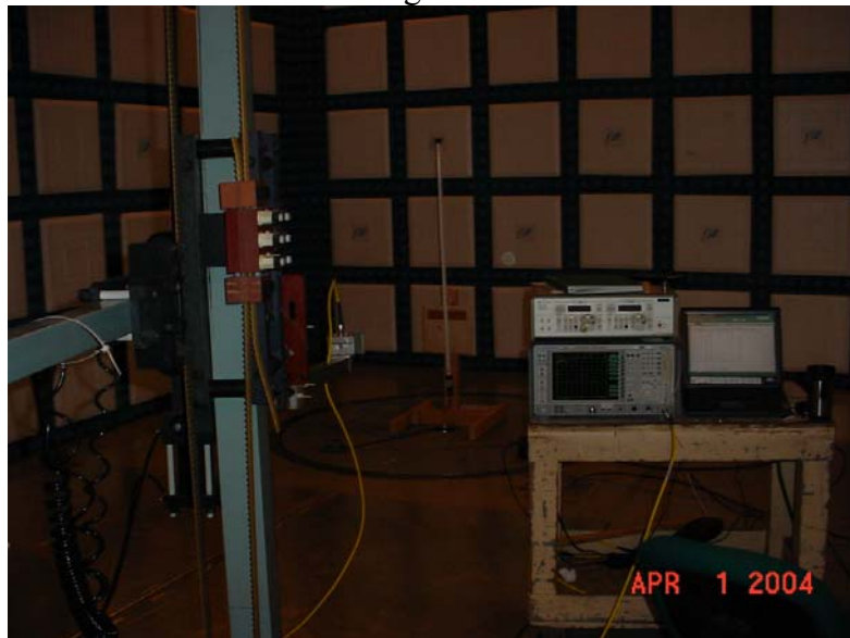
Test Setup for Measurement of Radiated Emissions from a Comtelco Model BS2400XL12-0 Omni Antenna
