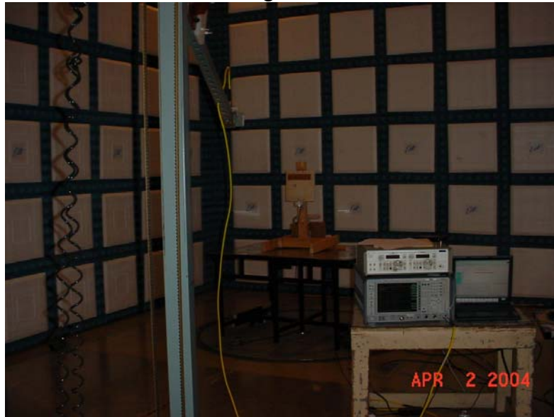
Test Setup for Measurement of Radiated Emissions from a WIFI MP5 Omni Antenna
