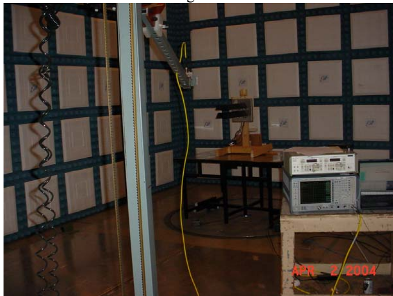
Test Setup for Measurement of Radiated Emissions from a WIFI Tetrad-M Array Antenna
