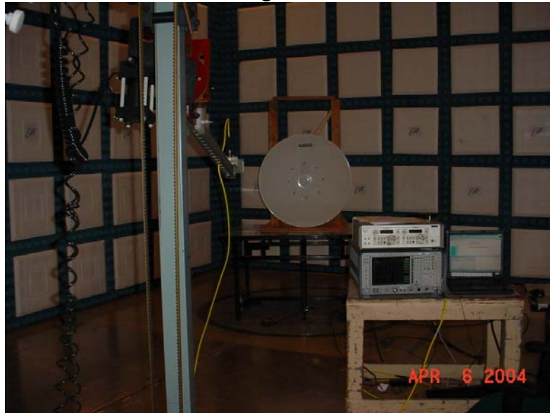
Test Setup for Measurement of Radiated Emissions from MaxRad Model MPR24026PTNF Dish Antenna
