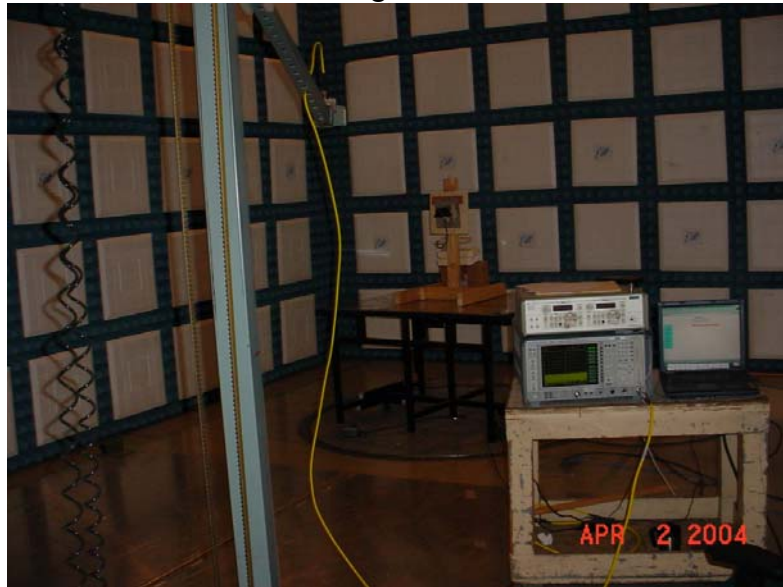
Test Setup for Measurement of Radiated Emissions from a WIFI Model MP 4in. Beam Antenna
