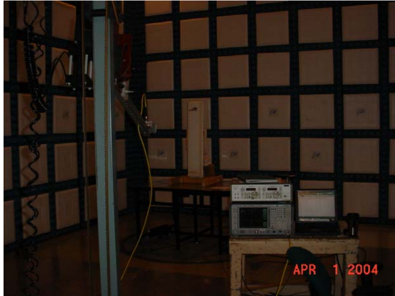
Test Setup for Measurement of Radiated Emissions from a RadioWaves 90° Sectored Antenna
