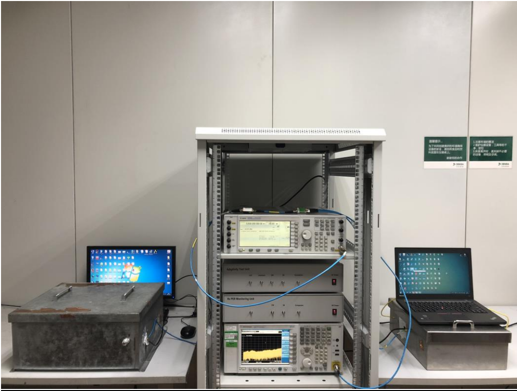
DFS Set-up Photo: Slave and Spectrum Analyzer
