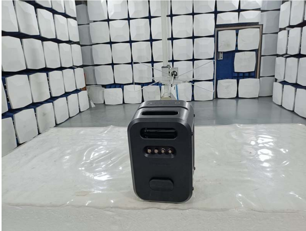
Radiated Emission Test Setup:
