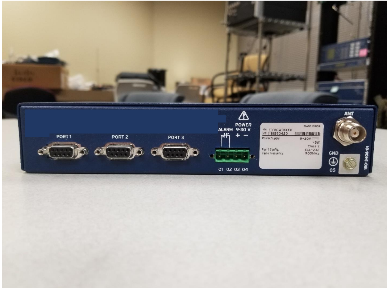
Figure 2: BACK - SERIAL PORTS, ALARM CONTACT, POWER INPUT
