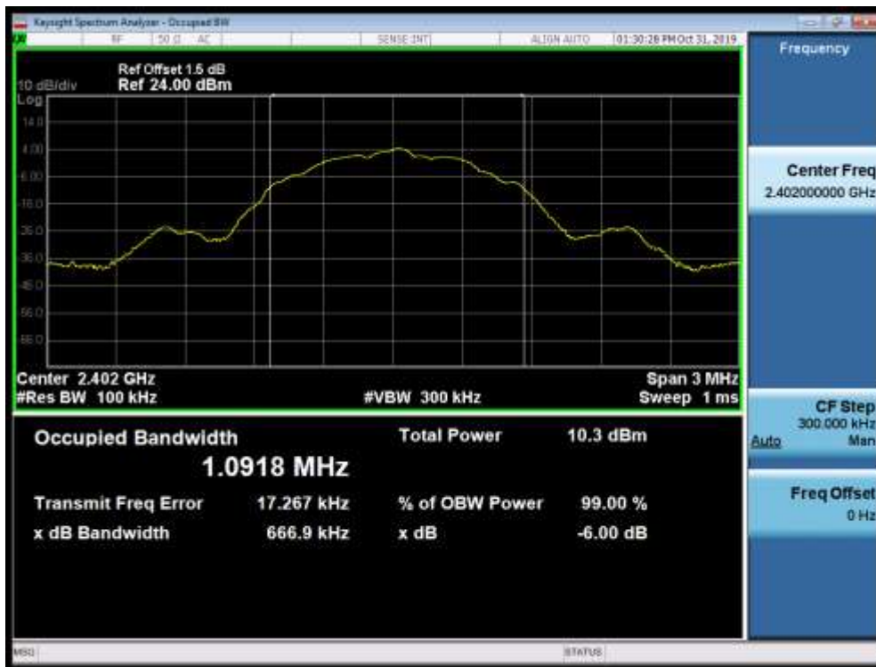
Mode 1 CH00 (2402MHz) for 6dB Bandwidth
