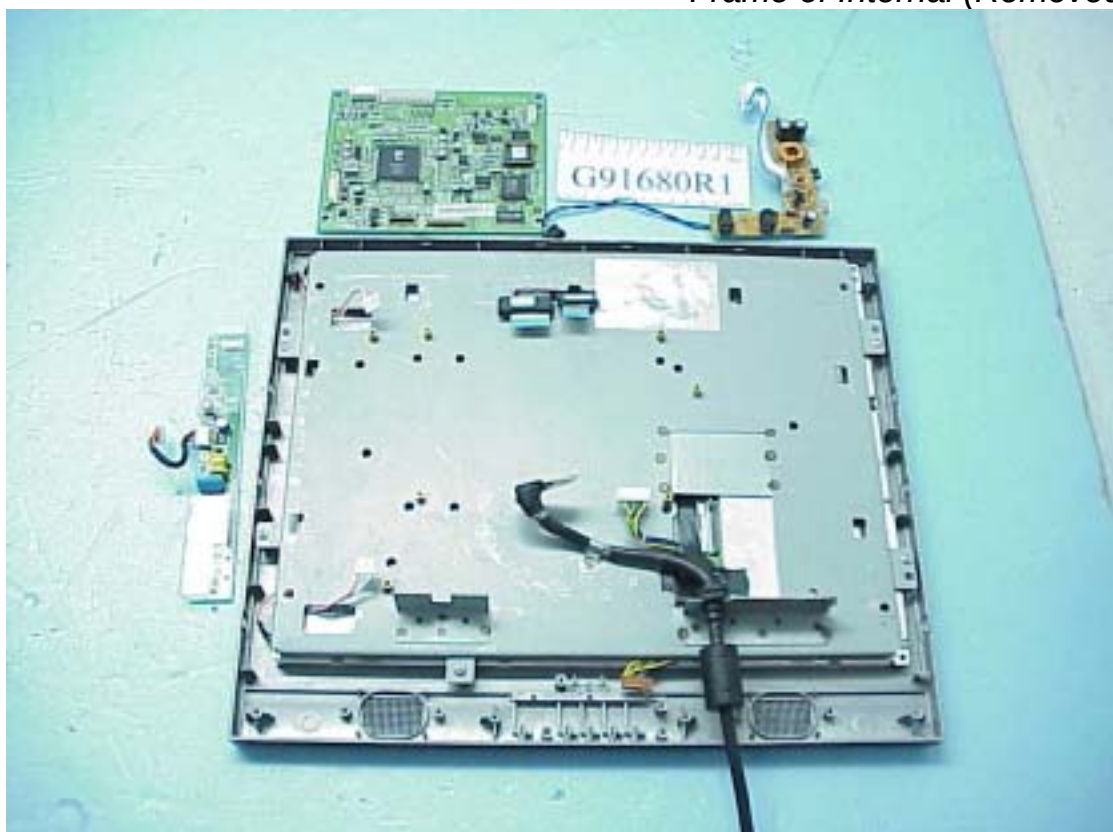
Figure 12 Frame of Internal (Removed PCB)
