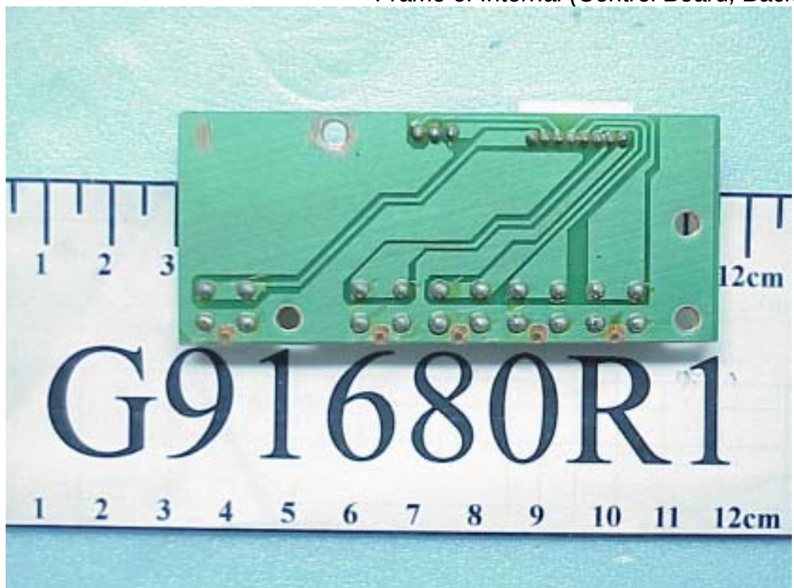
Figure 10 Frame of Internal (Control Board, Back Side)
