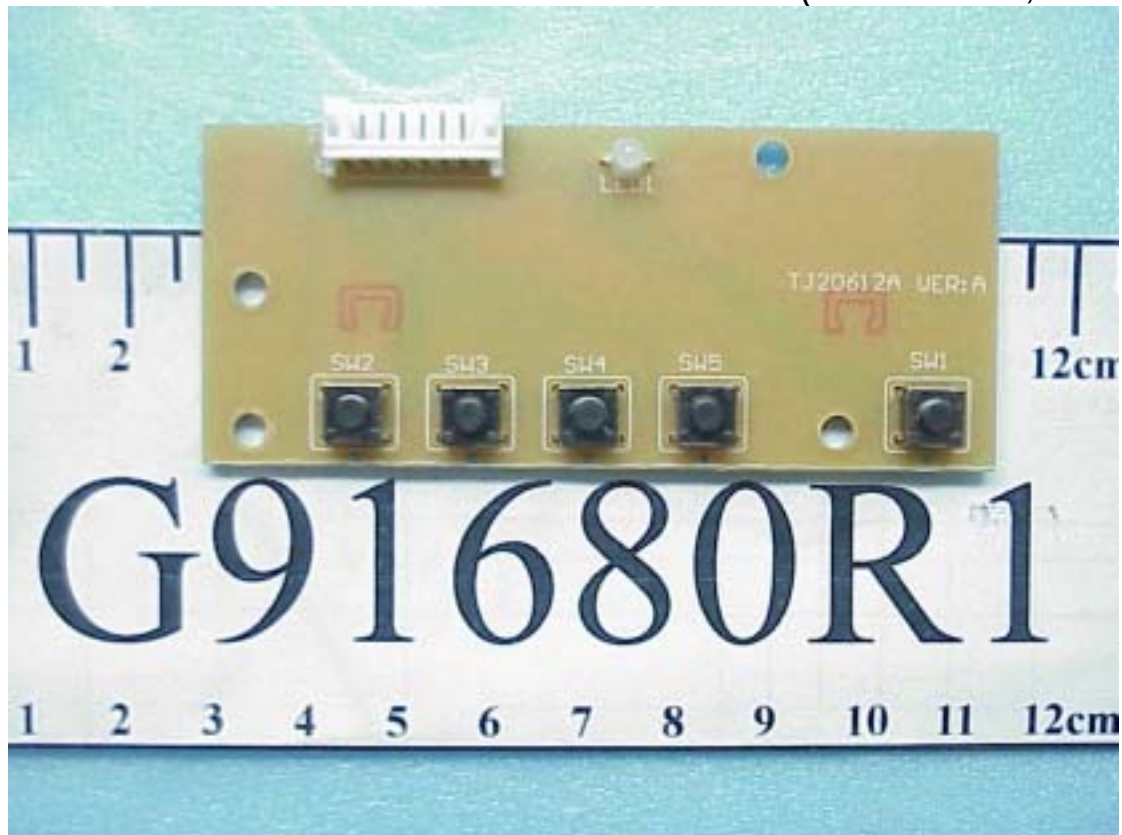
Figure 9 Frame of Internal (Control Board, Front Side)
