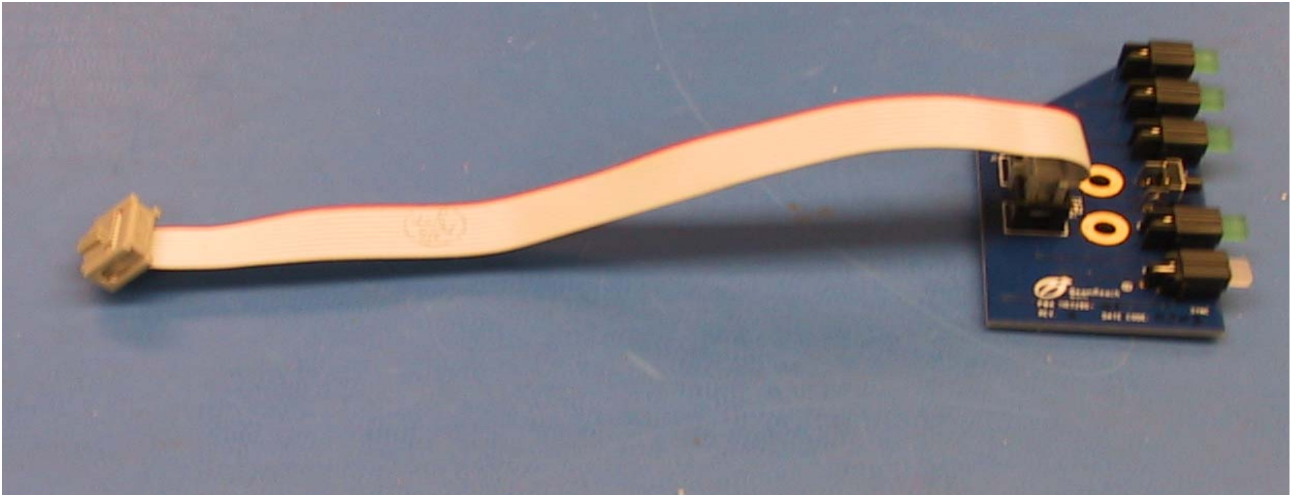
Figure 3. BRU-150, Front Panel LED Board and Cable.
