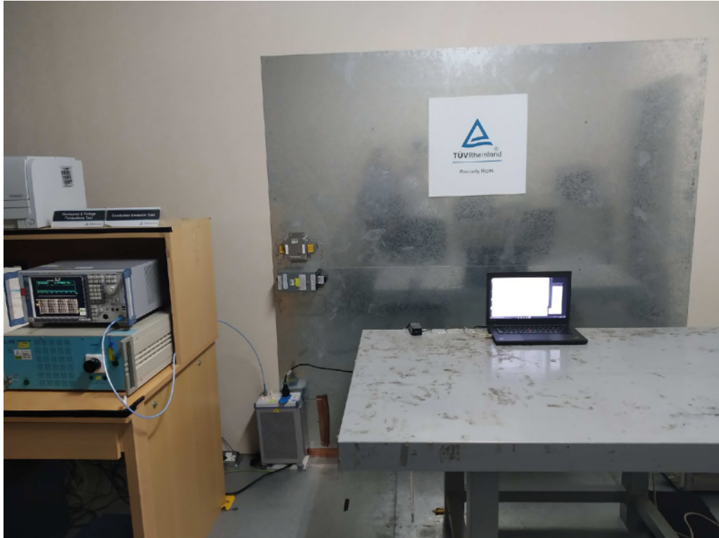
Photograph 9: Set-up for for Mains Conducted testing Front
