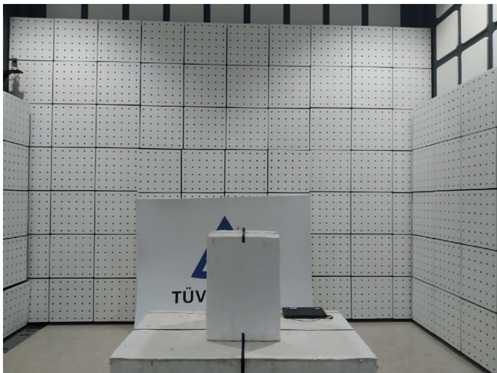
Photograph 2: Set-up for Spurious Emissions (Front View 2)
