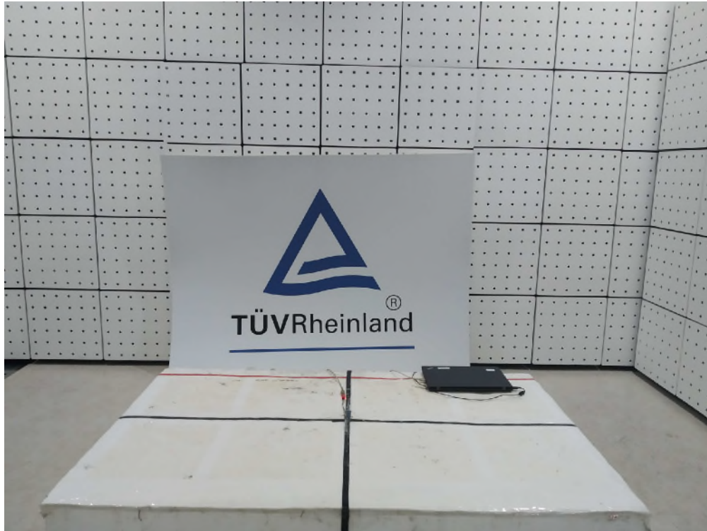
Photograph 1: Set-up for Spurious Emissions (Front View 1)
