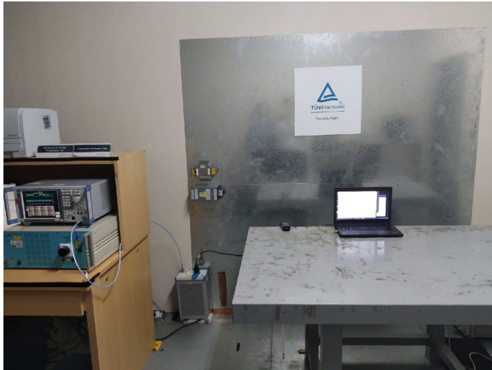
Photograph 8: Set-up for Mains Conducted testing (Front View)
