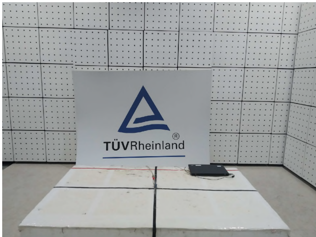
Photograph 1: Set-up for Spurious Emissions (Front View 1)
