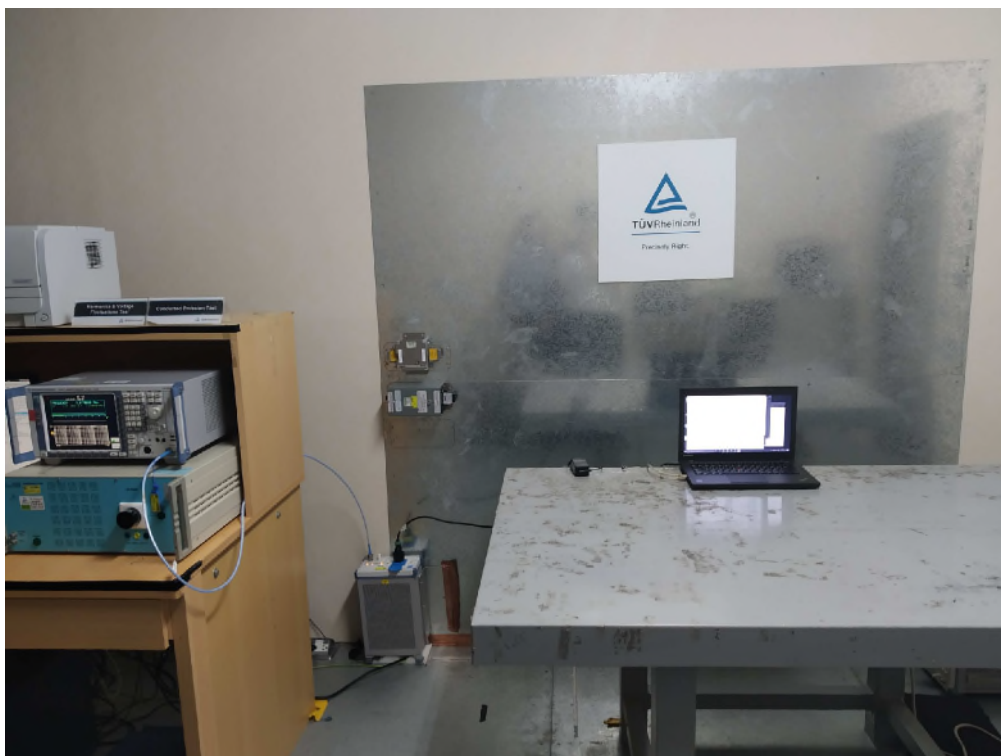
Photograph 7: Set-up for Mains Conducted testing (Front View)
