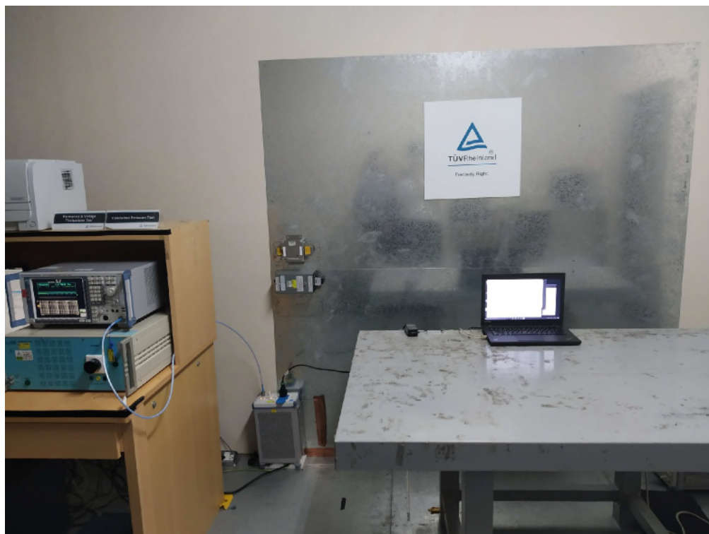
Photograph 7: Set-up for Mains Conducted testing (Front View)
