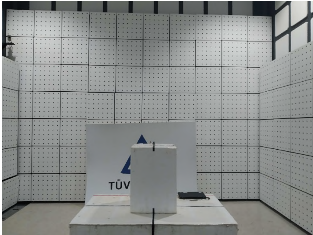
Photograph 2: Set-up for Spurious Emissions (Front View 2)
