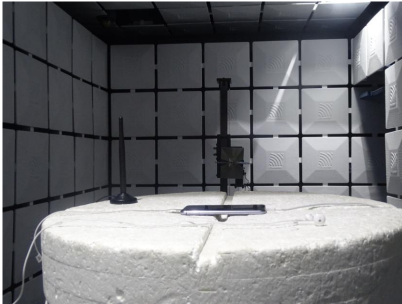
Radiated Spurious Emission (3GHz to 18GHz)
