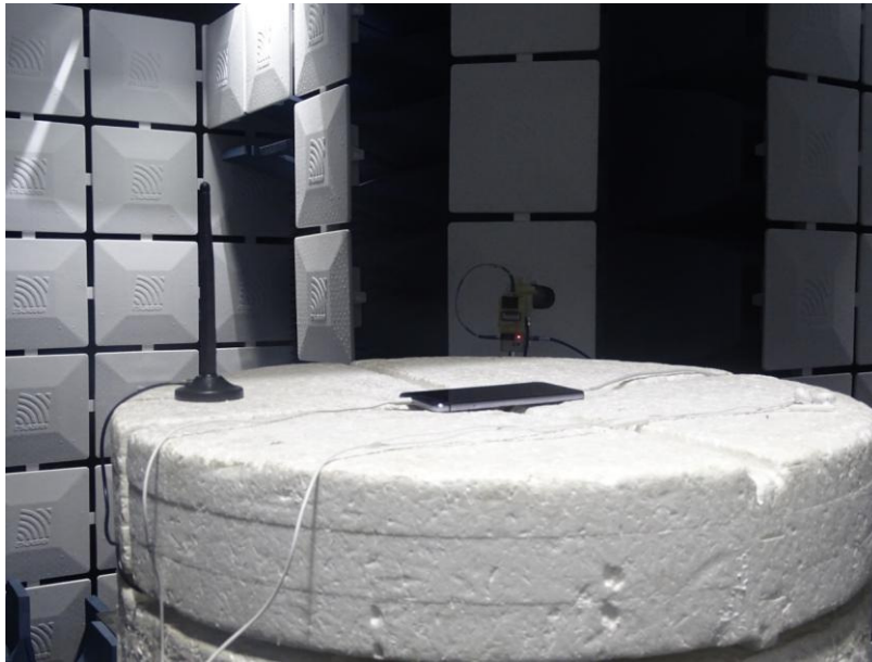
Radiated Spurious Emission (18GHz to26.5GHz)
