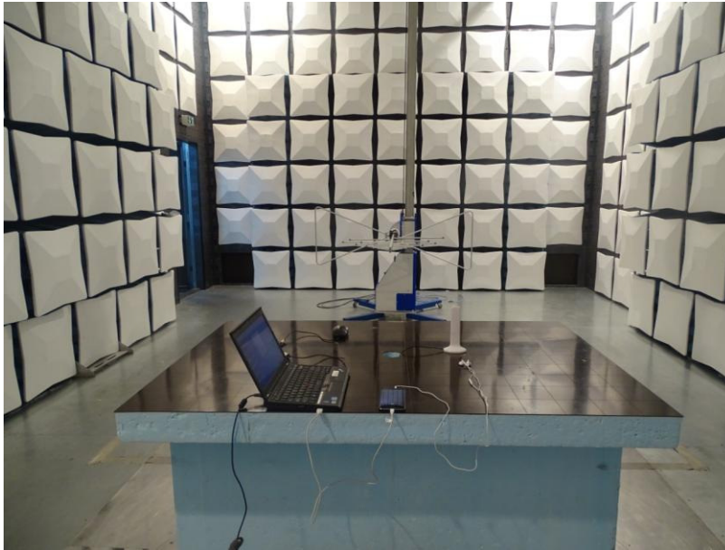
Radiated Spurious Emission (30MHz to 1GHz)
