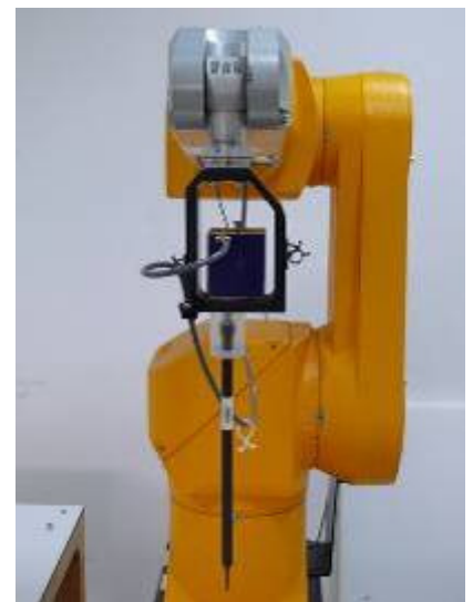
Figure 3. EX3DV4 E-field probe
