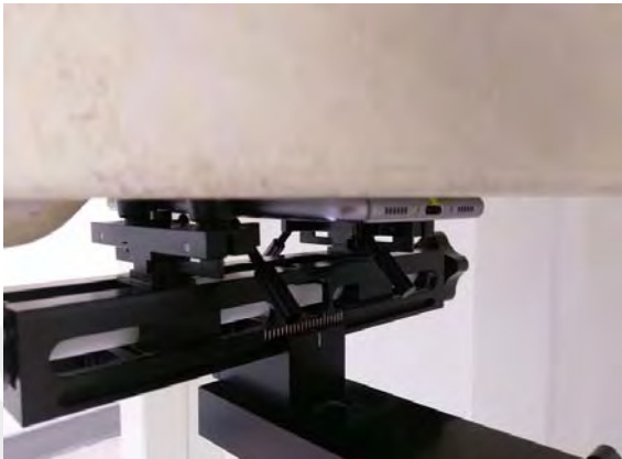
Fig.17 EUT Front side to flat phantom
