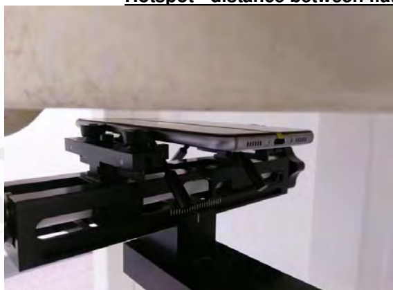
Fig.9 EUT Front side to flat phantom
