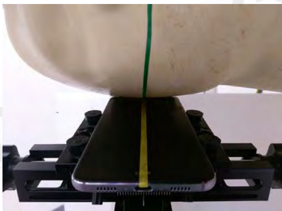
Fig.4 Right Head Section / Ear-Tilt Position(15°)
