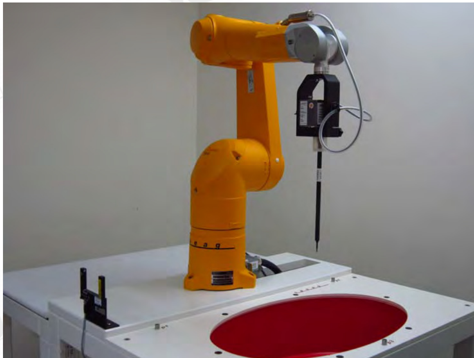
Fig.1 Photograph of the SAR measurement system
