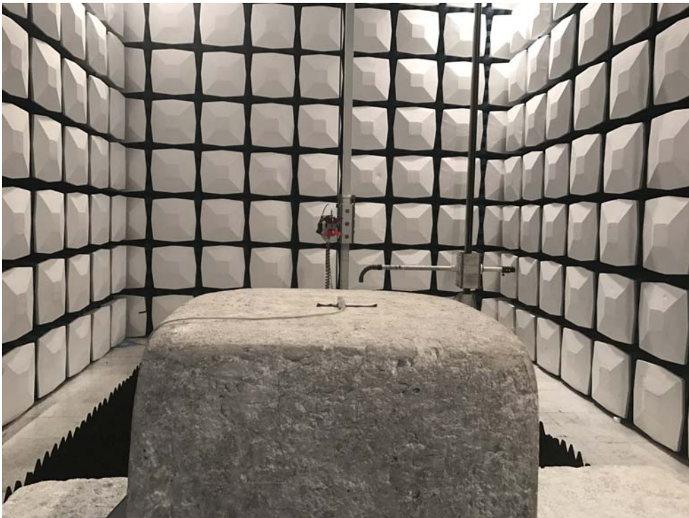
Description: Radiated Emission Test Setup for 1~18GHz
