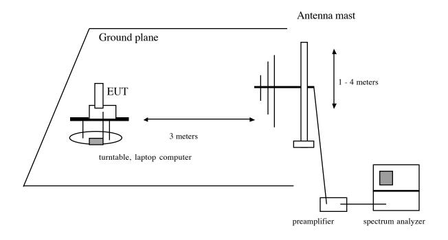
Radiated emissions generated by the digital portion of the EUT were measured.
