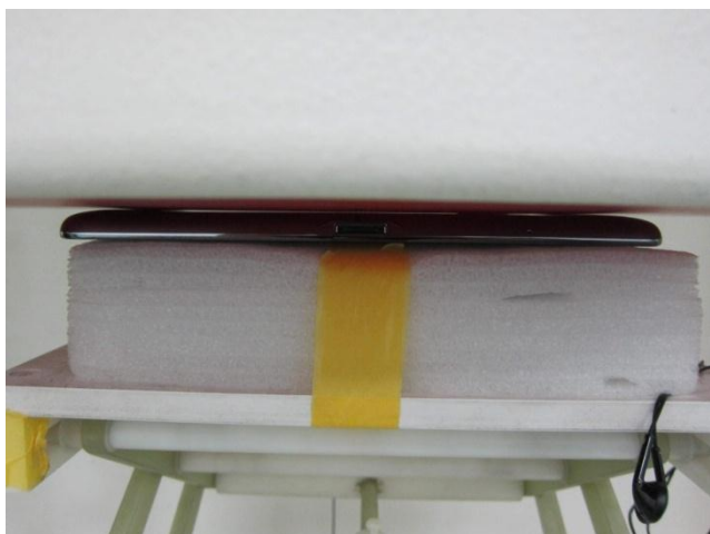
Bottom Face of EUT with earphone, 0cm Gap to the Phantom
