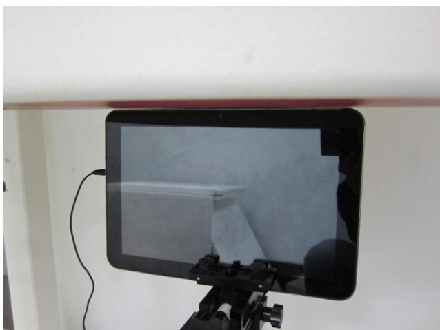
Secondary Landscape of EUT with earphone 0 cm Gap to the Phantom
