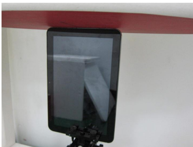
Primary Portrait of EUT with earphone 0 cm Gap to the Phantom
