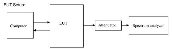
REMARKS: Attenuator loss (dB)=40dB, Cable Loss (dB)=1.5dB.
