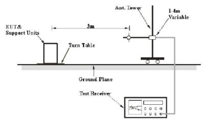
The radiated emission tests were performed in the 3-meter Chamber, using the setup accordance with the FCC part 2.1053. The specification used was the FCC 2.1053 limits.
