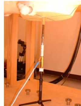
2450MHz System performance check setup
