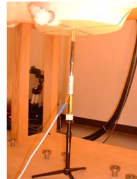
2450MHz System performance check setup
