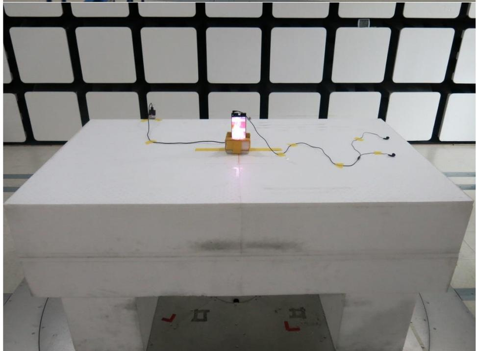
**Verification of Radiated Spurious Emissions at open-area test site
