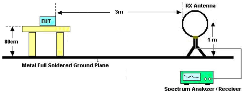
For radiated emissions from 30MHz to 1GHz
