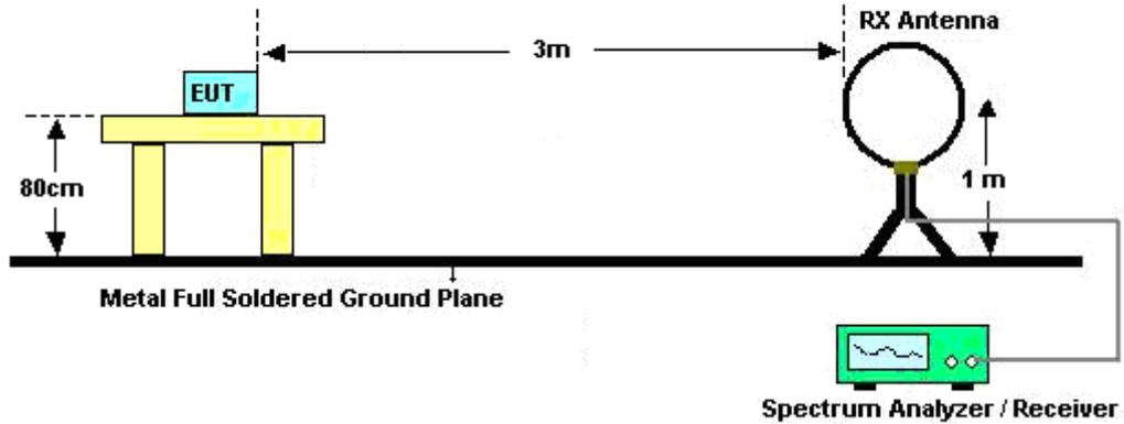
For radiated emissions from 30MHz to 1GHz
